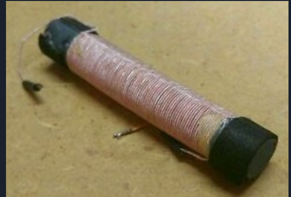
Figure 6: Ferrite rod antenna Inductance = 226\mu\text{H}
